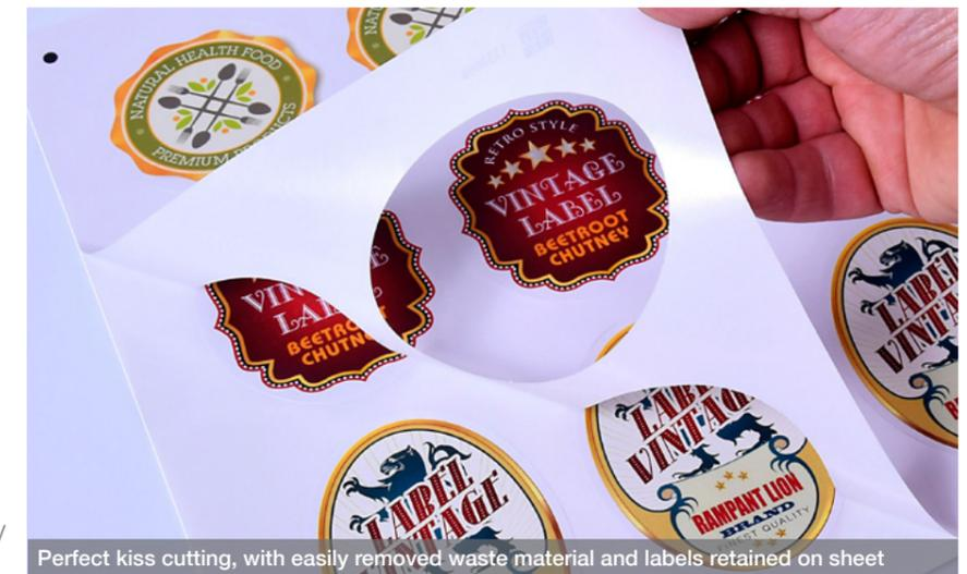
Perfect kiss cutting, with easily removed waste material and labels retained on sheet
